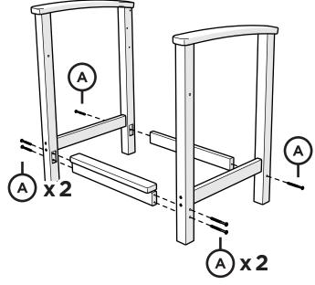
Do not tighten screws until last step.
