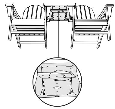
To lock in place, rotate SLIDE Lock forward.
