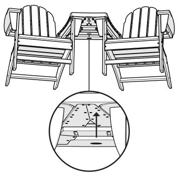
To lock in place, push SLIDE Lock forward.
