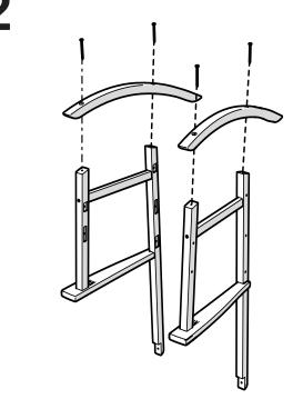
Partially thread each screw into pilot holes by hand before fully tightening.
