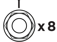
Flange Nylon Lock Nut HN.25-20FN
